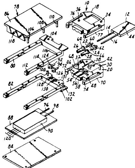
second elastomeric layer is mounted within the jack body beneath the first layer. The second layer both supports the split pin and exerts an upward compressive force on the first elastomeric layer.
